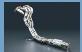
Exhaust Manifold (4-2-1 SUS type) 98,000yen For Racing (STD catalyst can't be installed)
