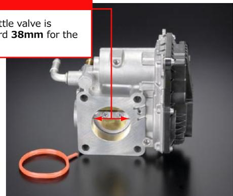
Increasing the diameter of the throttle and in combination with a tapered entrance helps to increase the amount of air the engine can breathe, giving improved performance. All parts are new. No trade-in is required so you get more performance and a new throttle assembly. By using with TODA light weight flywheel and light weight front pulley kit, you will experience a more sportier S660.
